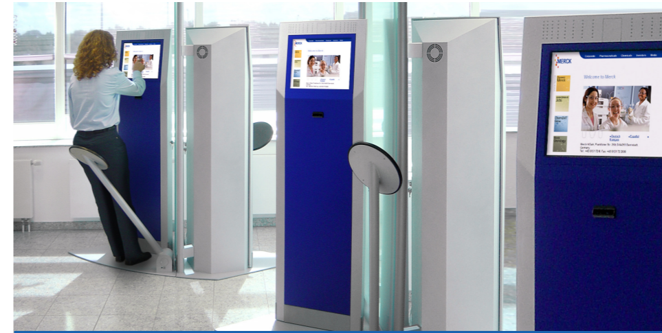
At Merck, sound showers are used to concentrate sound purely onto the person using the kiosk.
